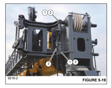
**9.** Attach the boom extension base section to the boom nose by installing the right side attachment pins through the anchor fittings and attachment lugs.
