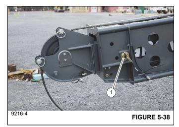
**5.** Pull the telescoping section out of the base section until the holes in the rear of the telescoping section align with the holes in the tip of the base section.
