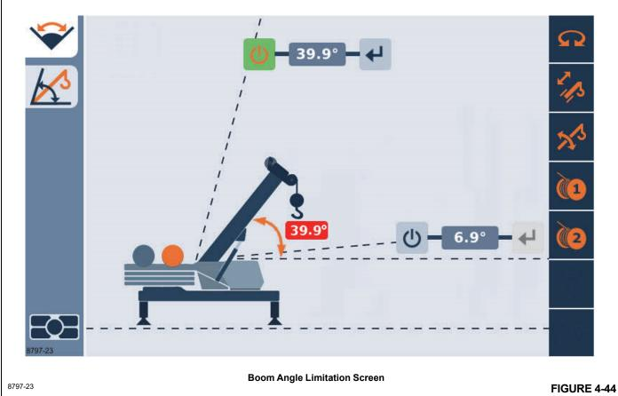
Using the Left Arrow and Right Arrow function on the Navigation Control Pad or the Jog Dial changes the object highlighted on the screen. As the arrow keys are pressed, the highlight will move between the objects, with the color orange typically meaning that the object is selected and can be affected by subsequent actions. In Figure 4-44, one can
