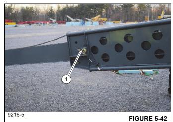
Using two people, slide the telescoping section into the base section until the holes in the front of the telescoping section align with the holes in the tip of the base section.
