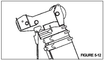
When anchoring socket to the boom, make sure flat face of socket is toward boom sections as shown in Figure 5-12.
