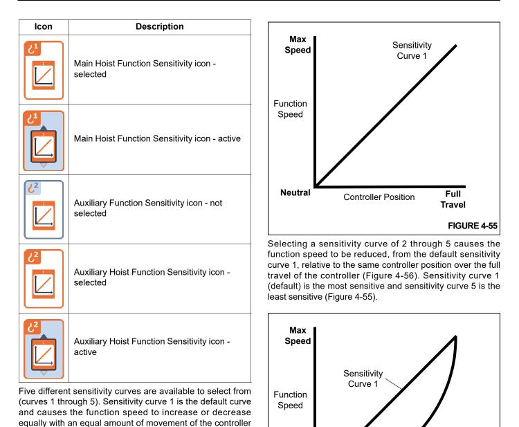
FIGURE 4-56 Adjust the sensitivity of a controller function by doing the following:
