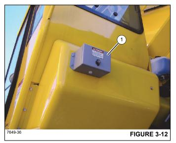
During maintenance or troubleshooting work, or to recover the crane, pressing and releasing the switch bypasses the following limiter systems and their crane function lock outs:
