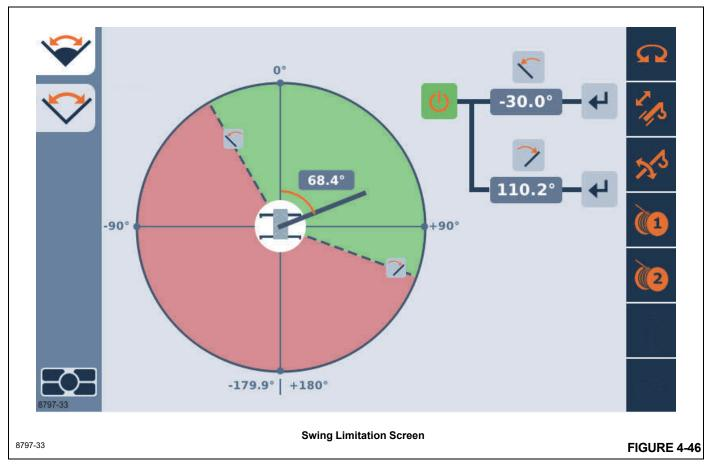
Using the Left Arrow and Right Arrow function on the Navigation Control Pad or the Jog Dial changes the object highlighted on the screen. As the arrow keys are pressed, the highlight will move between the objects, with the color orange typically meaning that the object is selected and can be affected by subsequent actions. In Figure 4-46, one can
