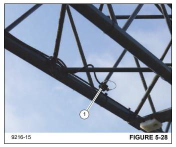
**c.** If the boom extension stinger section was <u>not</u> erected, disconnect the boom extension base section anti-two block cable end connector from the anti-two block switch at the nose of the boom extension stinger section. Stow the cable end connector in the stowage clip.
