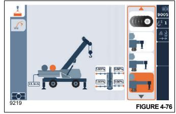
**3.** If required, use the Jog Dial or Arrow Buttons to select one of the following Boom Extension configurations (icon will turn orange) (Figure 4-77) and then press the Jog Dial or the OK Button to accept the selection.
