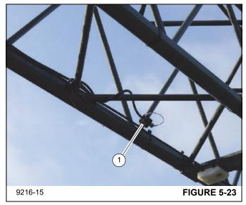
**b.** Disconnect the boom anti-two-block switch cable end connector from the anti-two-block switch at the boom nose and connect it to the boom extension anti-two-block cable end connector (1, Figure 5-24).
