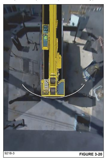
Birdseye View with Outrigger Pad Target Overlay
