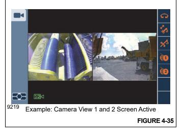
The active camera view is also displayed on the Main Screen of the ODM (Figure 4-36).
