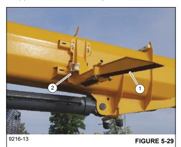
**9.** Disengage the attachment pins securing the left side of the boom extension to the boom nose.
