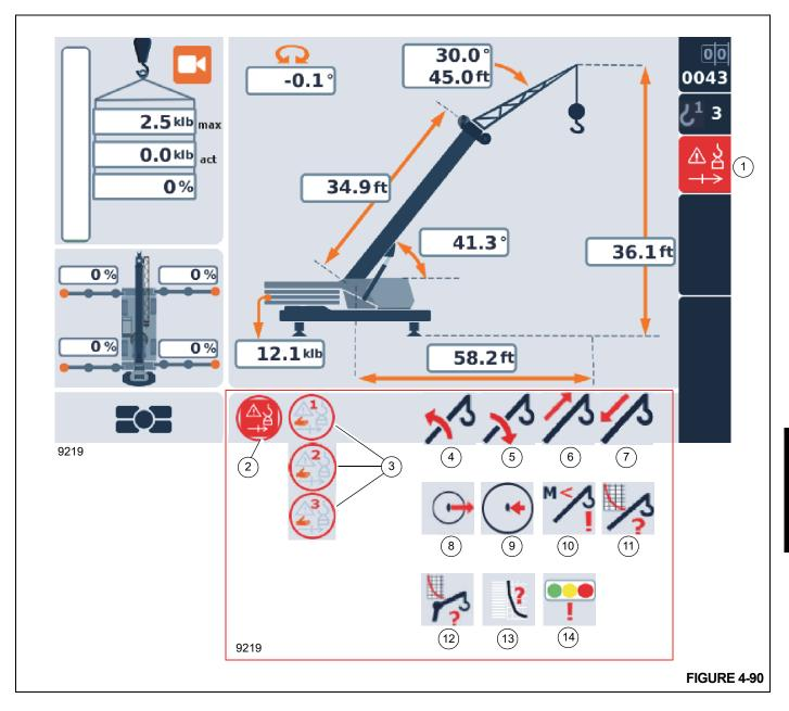
The following indicators can appear at the bottom of the Main Screen of the RDM (Figure 4-90)
