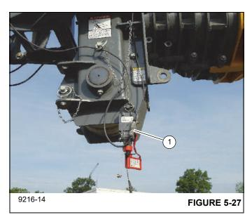
b. Wrap the boom extension anti-two block cable around the boom extension lacing, then secure the anti-two block cable end connector in the stowage clip (1, Figure 5-28)
