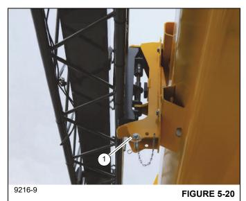
**11.** Disconnect the boom extension from the front stowage bracket by using an impact wrench and the provided extension (80104116) and socket (80104383) to turn the jack screw counterclockwise (1, Figure 5-21).
