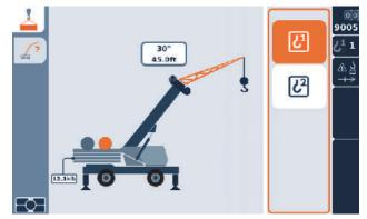
Example of On Outriggers and Boom Extension Erected 9219 FIGURE 4-81
