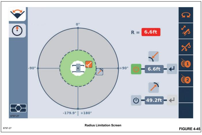
Using the Left Arrow and Right Arrow function on the Navigation Control Pad or the Jog Dial changes the object highlighted on the screen. As the arrow keys are pressed, the highlight will move between the objects, with the color orange typically meaning that the object is selected and can be affected by subsequent actions. In Figure 4-45, one can
