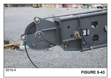
**7.** Connect the boom extension stinger section anti-two-block cable end connector to the anti-two-block switch at the nose of the boom extension stinger section.
