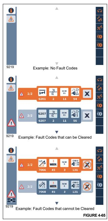
Crane fault codes with an "X" beside them can be cleared by the operator. Crane fault codes with an "X" surrounded by a red circle with strike-through cannot be cleared without first
