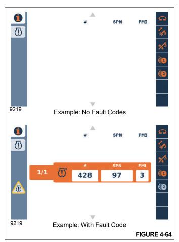
If several fault codes are active, use the Jog Dial or Arrow Buttons on the Navigation Control Pad to select the arrow at the top or bottom of the screen to scroll through the codes
