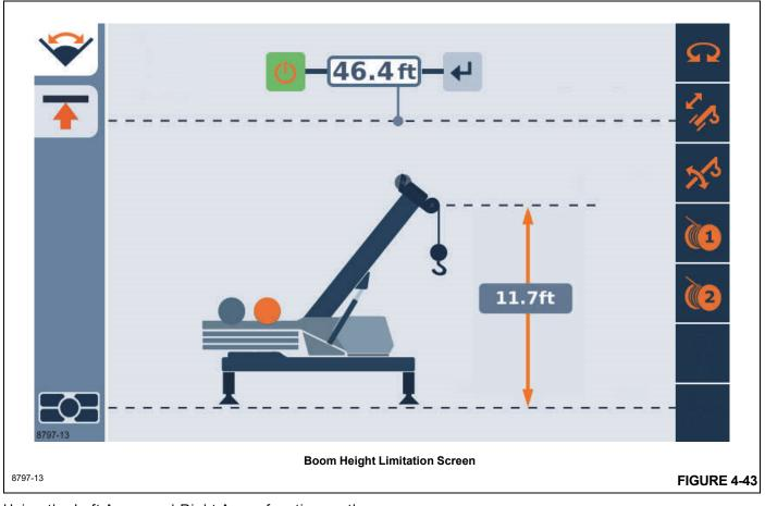
Using the Left Arrow and Right Arrow function on the Navigation Control Pad or the Jog Dial changes the object highlighted on the screen. As the arrow keys are pressed, the highlight will move between the objects, with the color orange typically meaning that the object is selected and can be affected by subsequent actions. In Figure 4-43, one can
