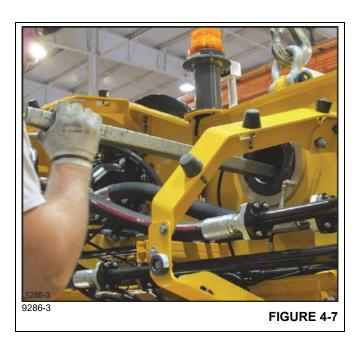
Reach in access hole at top of boom, install pins on stop plates already installed on back of mounting pins (Figure 4-8).
