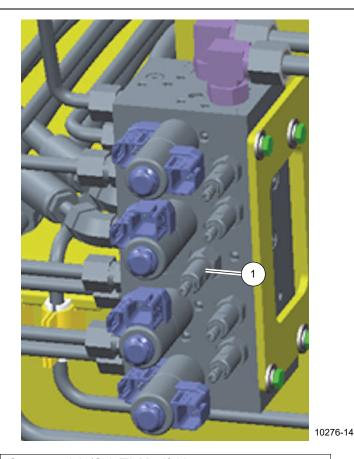
Counterweight/Cab Tilt Manifold
