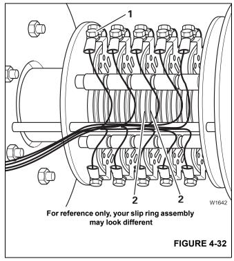
Remove visible dirt on the slip rings (2), (Figure 4-32) with a clean, lint-free cloth.
