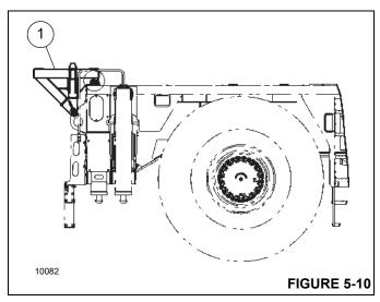
3. Rotate superstructure 90° for clear access to rear deck.
