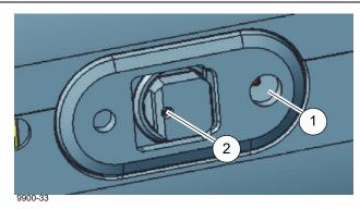
BOOM SERVICE LOCATIONS – REAR UPPER WEAR PADS AND LOCKING PINS
