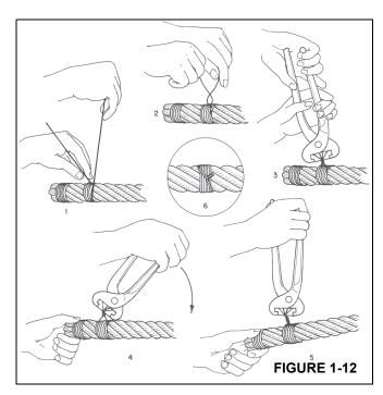
Wind a length of soft annealed wire (Figure 1-12) around the wire rope at least seven times. The two ends should be twisted together in the center of the seizing. Tighten the seizing by alternately prying and twisting. Cut off both ends of the wire and pound the twist flat against the rope.
