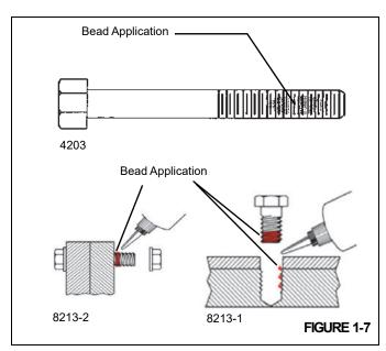
After application and engagement of mated threads, fixturing will occur within five (5) minutes. Time required to achieve full strength is 24 hours.
