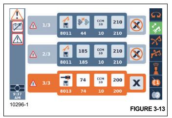
Fault codes with an "X" beside them can be cleared by the operator. Fault codes with an "X" surrounded by a red circle with strike-through cannot be cleared without first correcting the malfunction, then cycling the ignition key to the Off position and back to the On position.
