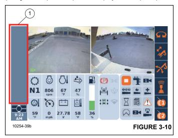
The Engine Fault Active Alert comes on when an engine or transmission fault is present, and the Crane Fault Active Alert comes on when a crane function fault is present (Figure 3-11).
