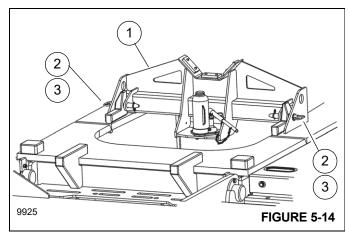
Remove the lift cylinder support (1, Figure 5-14) from the counterweight platform as follows:
