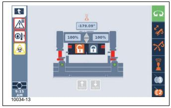
c. The lift cylinders raise the counterweight up to the superstructure. The lift cylinder icons turn green and the percentages show 0% when the cylinders are fully installed.
