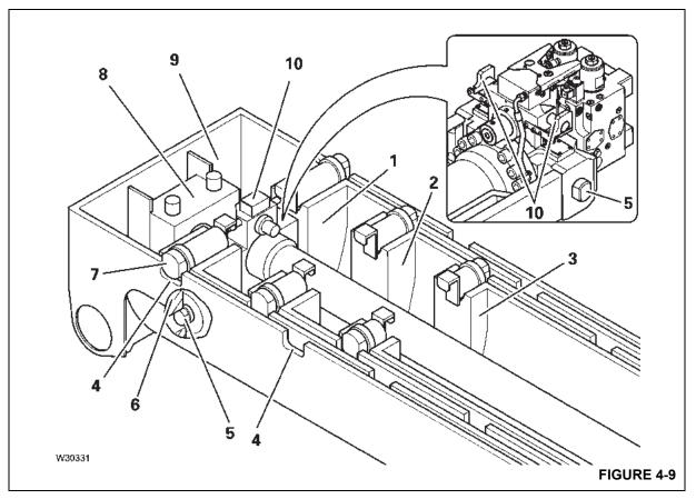
Each telescopic section is equipped with two section locking pins (7) which are extended by spring force.
