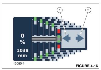
You can regulate the telescoping speed by moving the controller or changing the engine speed.
