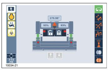
**13.** Using the ODM navigation control pad or jog dial, highlight the lock icon ♠. Press and hold the OK button on the ODM navigation control pad or the jog dial until the locking pins are locked (green).
