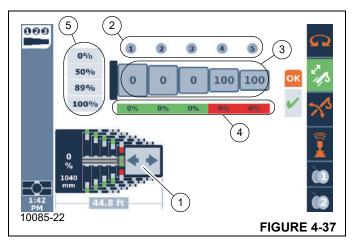
The arrows (1, Figure 4-37), at some point in the telescoping process, will blink. The blinking is an indication that an unlocking or locking event will occur if the operator holds the joystick in the direction of that arrow for at least 1 second. If this event begins, then the screen will change to the dots (as described for Figure 4-36) so that the operator knows that an automated motion or action is again occurring.
