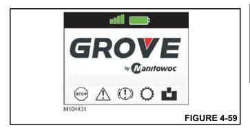
**11.** Press the Engine Button on the Remote Control Unit. The Engine Screen appears in the display.
