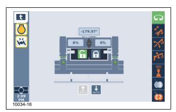
11. Using the ODM keypad or jog dial, highlight the down arrow . Press and hold the OK button on the ODM navigation control pad or the jog dial down until the counterweight cylinders are fully extended.
