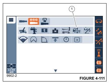
The Suspension Raise/Lower function screen (Figure 4-112) is used to lower and raise the crane suspension.
