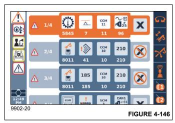
Crane fault codes with an "X" beside them can be cleared by the operator. Crane fault codes with an "X" surrounded by a red circle with strike-through cannot be cleared without first correcting the malfunction, then cycling the ignition key to the Off position and back to the On position.
