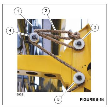
**19.** In the ODM, highlight the lock icon and the extend the rear boom extension pin (Pin #1) as follows:
