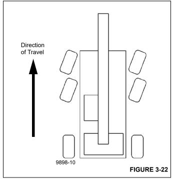
Push and hold the left side of the Rear Steer Switch to cause the wheels on the rear tandem axles to turn left, causing the crane to turn left as shown in Figure 3-23. Release the switch when the rear wheels are pointed in the desired direction.
