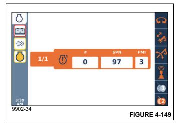
If several fault codes are active, use the Jog Dial or Arrow Buttons on the Navigation Control Pad to select the arrow at the top or bottom of the screen to scroll through the codes
