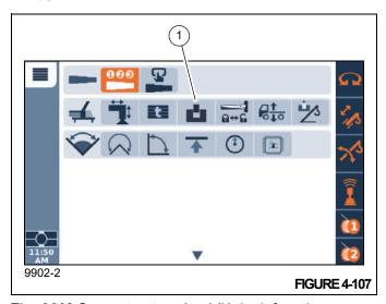
The 360° Superstructure Lock/Unlock function screen (Figure 4-108) is used to lock the superstructure in position any where throughout its 360° rotation.
