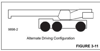
The Steering Reversal Switch is used to reverse the driving controls when changing between Standard Driving Configuration and Alternate Driving Configuration.
