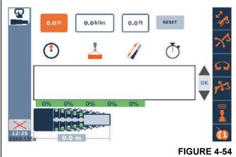
After a table of boom configurations is displayed, the arrow icons on the right side of the screen can be used to highlight a particular row in the table. For this highlighted row, the details of the boom configuration ("tele picture") is shown below the table. If the OK button is pressed with a particular row highlighted, then the boom configuration is sent directly to the Semi-auto screen and the control system begins to work that selection and can begin unlocking the boom.
