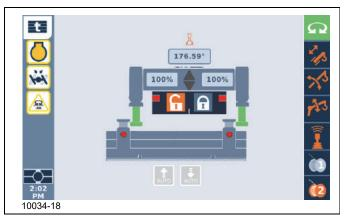
**NOTE:** The Up and Down counterweight cylinder arrows are active when the superstructure slew angle is between 179.5° to -179.5°.
