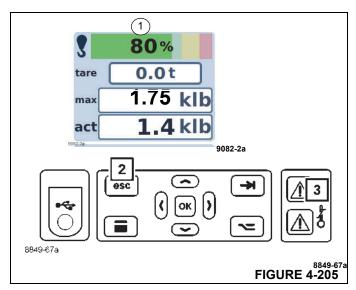
**NOTE:** If the capacity continues to increase, the RCL will reach an overload state and a RCL shutdown will occur.
