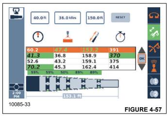
Finally, if it is desired to keep lifts within a criterion such as 75% of the maximum values for the load chart data, then the search can be based on a modified hook load. The modified hook load value would be the hook load divided by the decimal value for the desired limitation such as the following:
