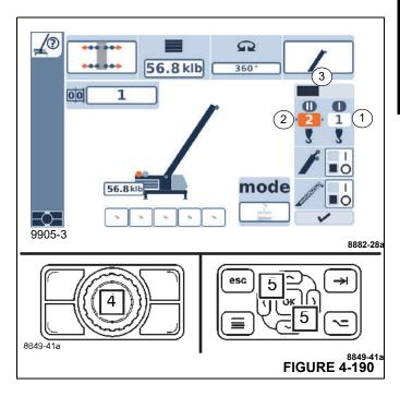
Position the slider bar (3, Figure 4-190) over the top of the hoist that is to be used. Example screenshot in Figure 4-190 shows the Auxiliary Hoist is selected.
