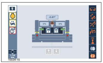
NOTE: The superstructure must be slewed between 179.5° to -179.5° to activate the counterweight cylinder Up and Down arrows (8, Figure 5-16).
