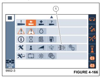
The Exhaust System Cleaning function screen (Figure 4-167) allows the operator to initiate or inhibit the exhaust system cleaning process.
