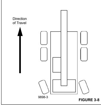
NOTE: When driving the crane with the boom centered over the rear tandem axles, the steering axle and wheels are behind the operator. Thus, the operator must become familiar with the steering characteristics of a rear-steering axle, including the tail-swing of the crane, before driving the crane at higher speeds and around obstacles.
