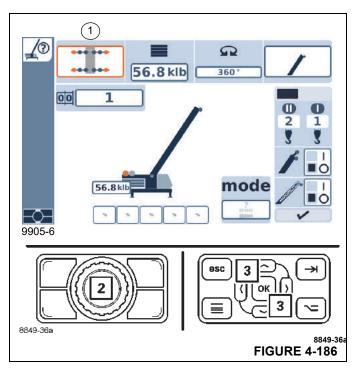
The outrigger span is monitored when outrigger monitoring is installed. You must check the outrigger span when entering the rigging mode.
