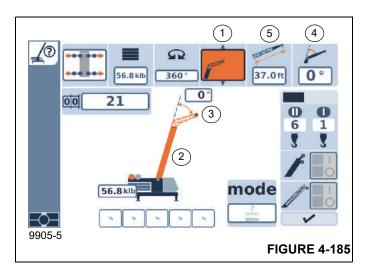
Use symbol (1, Figure 4-185) to select the rigged boom system.
