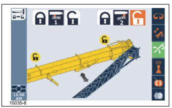
16. Visually confirm that the front mounting pin (Pin #2 in the ODM) is unlocked. The handle should be in the down position. When the handle is in the down position, the front mounting pin is retracted and the boom installation pins are locked.
