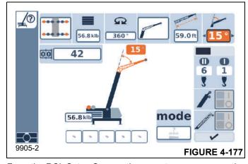
From the RCL Setup Screen, the operator can program the RCL either by entering a rigging code number from the *Load Chart Manual* or by entering the crane configuration using the setup wizard
