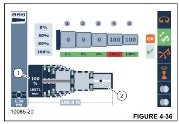
The example in Figure 4-36 shows the value of 10571 mm for the extension of the telescoping cylinder within the boom. This is the value from the precision length sensor. The example also shows a value of 108.8 feet as the overall boom length. The example shows the T5 boom section had been previously extended and locked at its 100% pinning location and the T4 boom section is being pinned at the 100% pinning location. The remaining boom sections are locked at their 0% pinning location.
