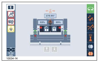
**d.** The locking pins are extended. The locking pin icons turn green when the pins are fully extended.
