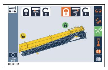
**16.** Make sure the ODM shows that the front mounting pin (Pin #2) is extended. Visually confirm that the front mounting pin is securely installed. Lock the handle (1, Figure 5-38) with pin (2).
