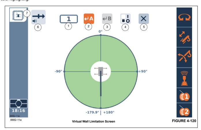
The Virtual Walls Limitation Menu allows the operator to define up to five walls or barriers in which the boom is not expected to operate.
