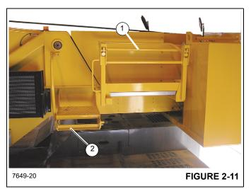
Use the hoist access platform (1) (Figure 2-12) when working in the hoist area (Fixed counterweight units only).
