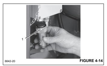
**c.** Install cable end connector (1) Figure 4-15 from boom extension where dummy plug was removed.
