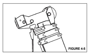
When anchoring the socket to the boom, ensure the flat face of the socket is in position, as shown, toward the boom sections (Figure 4-5).
