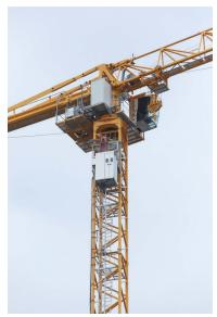
Chantiers de l'Atlantique added a MDT 389 L12 on basin C to increase the productivity of the manufacture of large cruise ships. To protect the crane from the effects of salt water and the harsh environment close to the sea, the crane was delivered with a high durability paint system with metallization.
