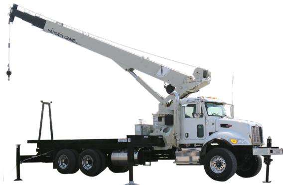
The H Series models have multi-position outriggers that offer excellent setup flexibility for job site conditions. The Rated Capacity Limiter (RCL) displays the actual outrigger setup, crane configuration and diagnostic information.
