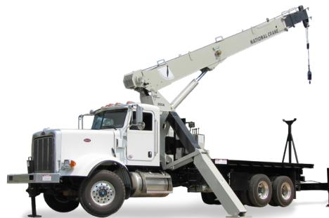
National Crane offers the broadest range of telescoping cranes with stand up controls. Capacities range from 10 USt – 33 USt (9,1 t – 29,9 t), and National Crane boom trucks have the most available options and mounting configurations on the market.
