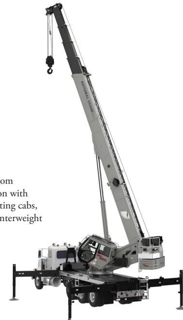
National Crane takes the boom truck into the next generation with advanced features such as tilting cabs, hydraulically removable counterweight and unmatched capacities.
