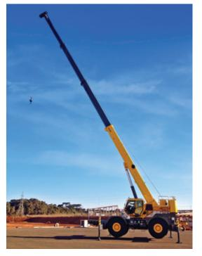
Synchronized boom telescoping allows each boom section to be extended simultaneously with a single-lever control.
