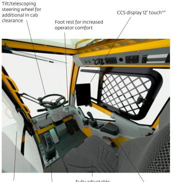
Sliding side and rear tinted windows Fully adjustable heated seat (front, back and vertical)
