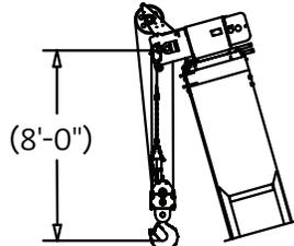
Dimensions are for largest furnished hookblock and headache ball with anti-two block activated.
