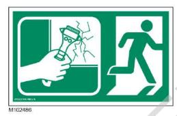
Using the life hammer provided, smash the front window to exit the operator cab in an emergency. The hammer is stored on the left wall inside the operator cab.
