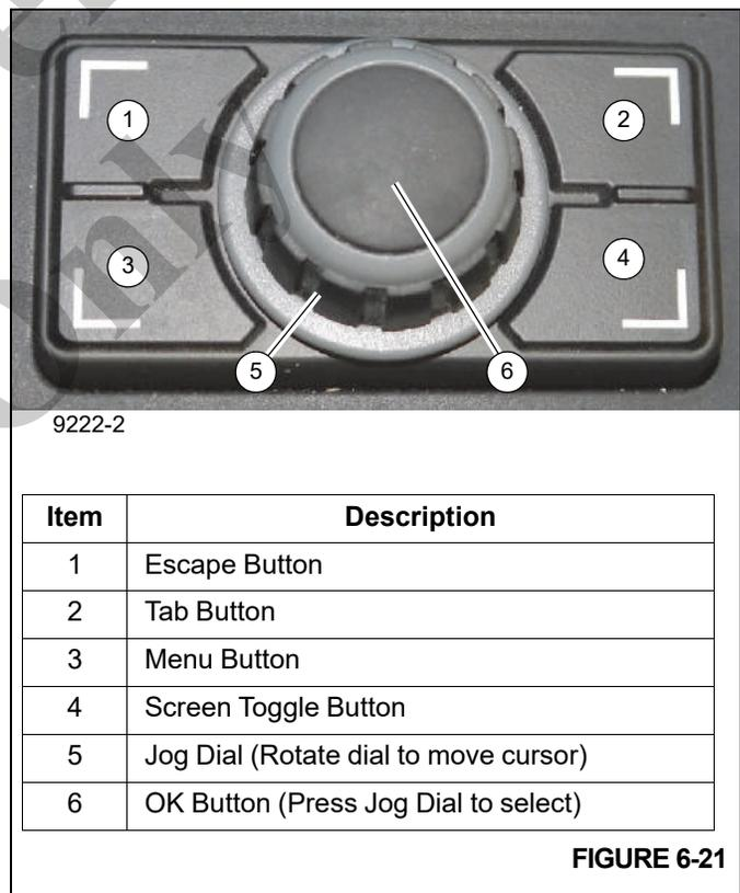
Upon selecting a camera view from the Menu Screen and pressing the Jog Dial or OK Button, the ODM will switch to the corresponding Camera View Screen (Figure 6-22).
