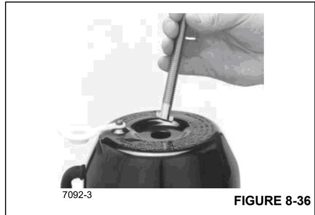
**NOTE:** If the items referred to in Steps 3 and 4 are not stored in/on the chamber, they must be obtained from the vehicle tool box or Manitowoc Crane Care, as the piggyback spring brake cannot be manually released without them. (Figure 8-35) shows the bolt external storage area.
