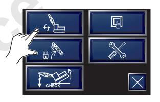
(3) Crane attachment select screen is displayed. Select "10 (Self removal mode)".
