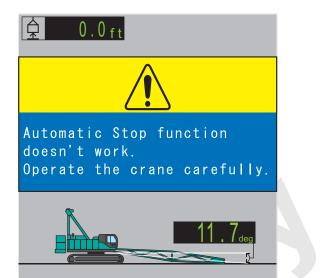
5. Stop release mode when transportation with boom base attached.
